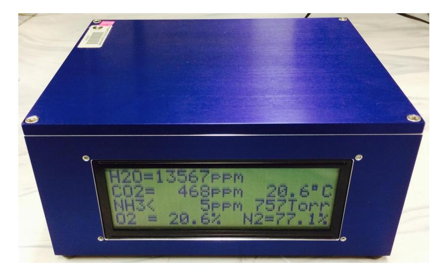
Mass: 2 Kg Vol: 3.1 L Power (120VAC/6VDC): 2.6W Data Log: 1 min averages
