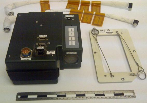
Mass: 2.6 Kg Volume: 4.4 L Power: 2.5 W • USB (5VDC) or • 28VDC or • Internal batteries Memory: 16 GB Data log: 30sec avg's
